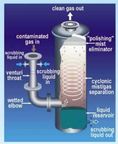
(Mainly for Particulate removal from boiler flue gas and Rotary Kiln exhaust gas)
