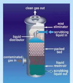
The Packed Tower Scrubber can be designed to any particular efficiency desired. Our engineers can select the type of packing, scrubbing liquid and tower size best suited to your particular needs.
