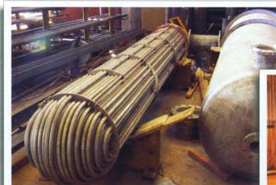
H.P. Heater under fabrication for 40mw power plant.
